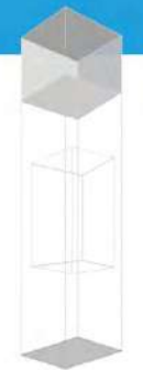
小机房电梯的机房 Machine room in small machine room elevator
